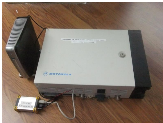
Pictured is PARA's new Motorola Brand D-STAR 444.750+ repeater and gateway computer.
